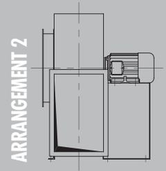
Impeller directly mounted on motor shaft and all mounted on full depth pedestal.
